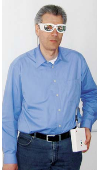
Figure 1.3: The Learning Retinal Implant from Intelligent Medical Systems. It is designed to help patients with retinitis pigmentosa. The eye glasses and photoprocessor worn on the waist are used to train the retinal implant, thus restoring vision [5].
