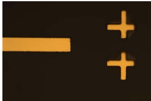
Figure 6.5: 1.0 \mu\text{m} thick coil trace with good resolution. Outline is sharp and free of excess gold.
