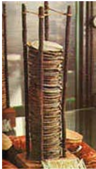
Figure 2.8: Voltaic pile consisting of a series of alternating zinc and copper disks separated by cardboard soaked with an acid or salt solution [25]
